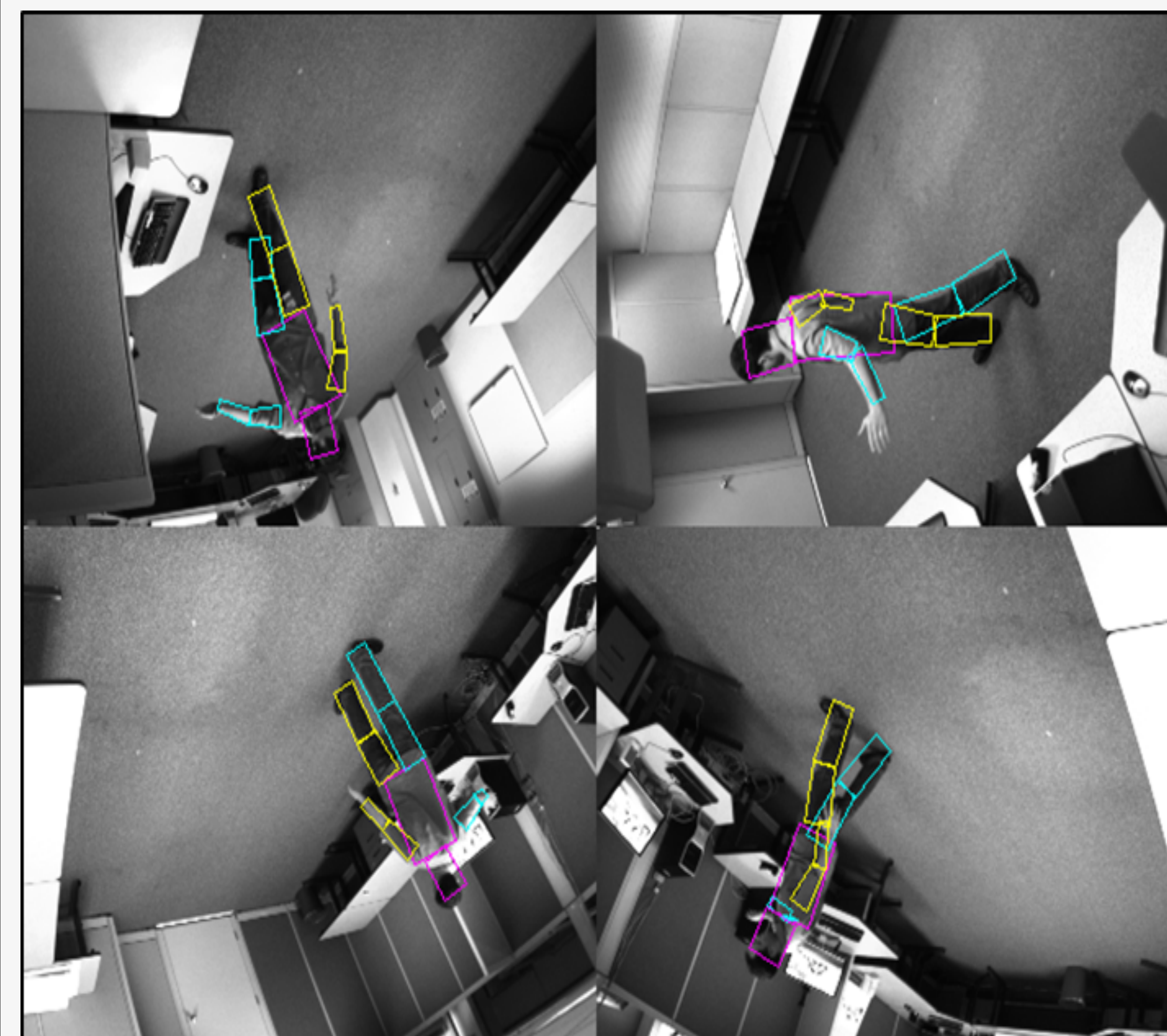
Figure 1 - Bodytrack is a computer vision application that tracks a human body. Above is the output of two different runs of Bodytrack, one using a precise architecture and the other using load value approximation. The similarity is uncanny, and approximating load values can save 44% in energy and improve performance by over 14%.
