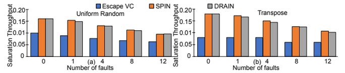
Figure 10: Saturation throughput for synthetic traffic patterns with increasing number of faults in an irregular  $8 \times 8$  mesh.
