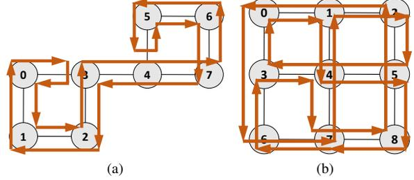
Figure 6: Sample outputs of our offline algorithm for (a) an irregular topology and (b) a regular topology. Each arrow represents a unidirectional link in the drain path.
