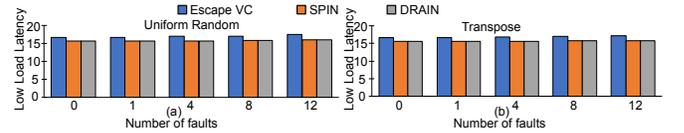
Figure 11: Low-load latency for synthetic traffic patterns with increasing number of faults in an irregular  $8 \times 8$  mesh.
