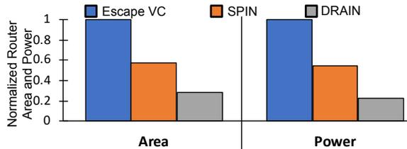
Figure 9: Router area and static power comparison.
