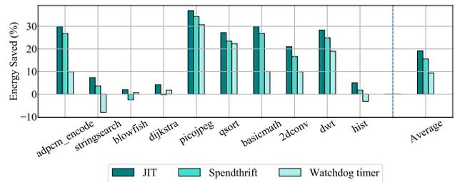
Figure 10: Energy saved in NvMR with different backup schemes compared to Clank
