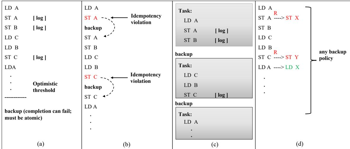
**Figure 2: (a) Backup policy with an optimistic threshold (backup must be atomic), (b) Clank (backup when there is an idempotency violation), (c) DINO (backup at the boundary of pre-defined atomic tasks), (d) NvMR (any backup policy of choice); R stands for renaming. NVM addresses A and B are renamed to X and Y.**
