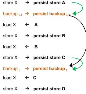
**Figure 4: Happens-before persist orderings with proposed NVM renaming. By renaming X, all stores access only write-dominated memory locations. Only the stores that immediately precede backups must be persisted.**
