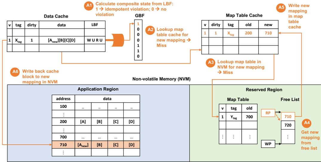
Figure 7: Eviction of a cache block with tag  $X_{tag}$  causes an idempotency violation. Cache block address 200 is renamed to address 710. The dirty cache block is stored at the new mapping 710 instead of 200.
