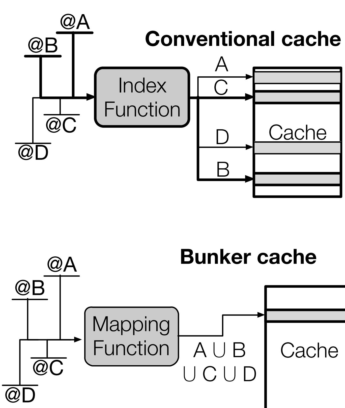
The Bunker Cache requires only modest changes to cache indexing hardware, integrating easily into commodity systems.
